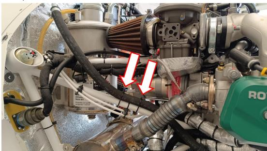
The oil hose is currently secured with two plastic zip ties. If the zip ties fail, the unsecured oil hose could shift and contact the nearby exhaust tube, potentially leading to a rupture or leak due to high temperatures.
