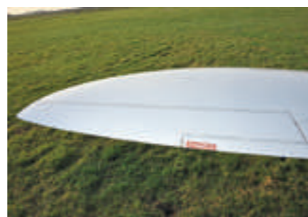
▲ Ailerons are made all the lighter by servo tabs
