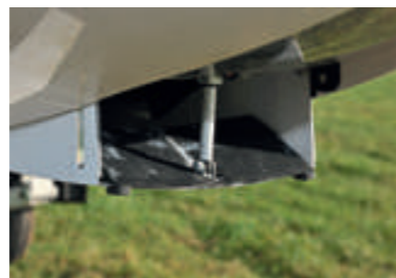
▲ Adjustable cooling intake: forget the usual trial-and-error blanking plates!
