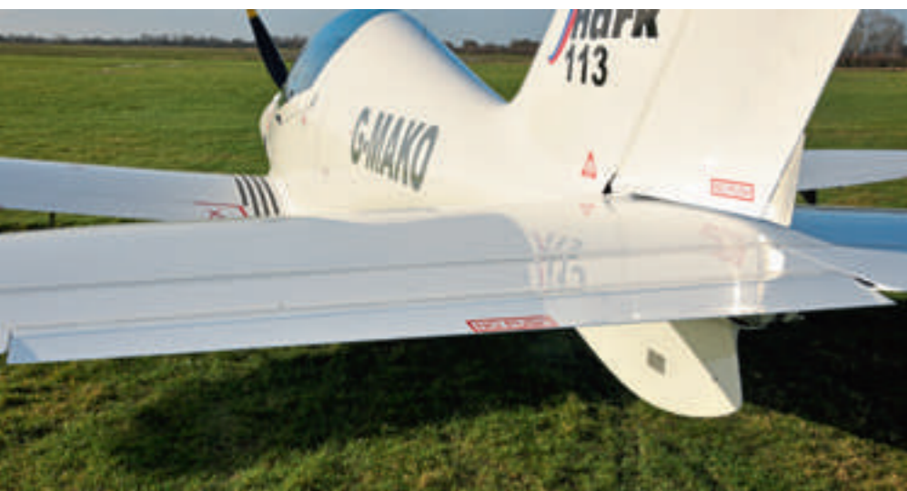
▼ Unusual refinements include the aerodynamic tweak of gap seals on all surfaces and a split elevator
