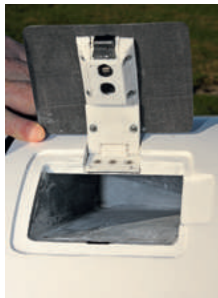
▲ With someone in the back seat, the supplied 6kg weight must be lodged in the cowl ballast box...
