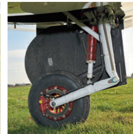
▲ Compliant trailing link main U/C legs have rubber-block spring/dampers
