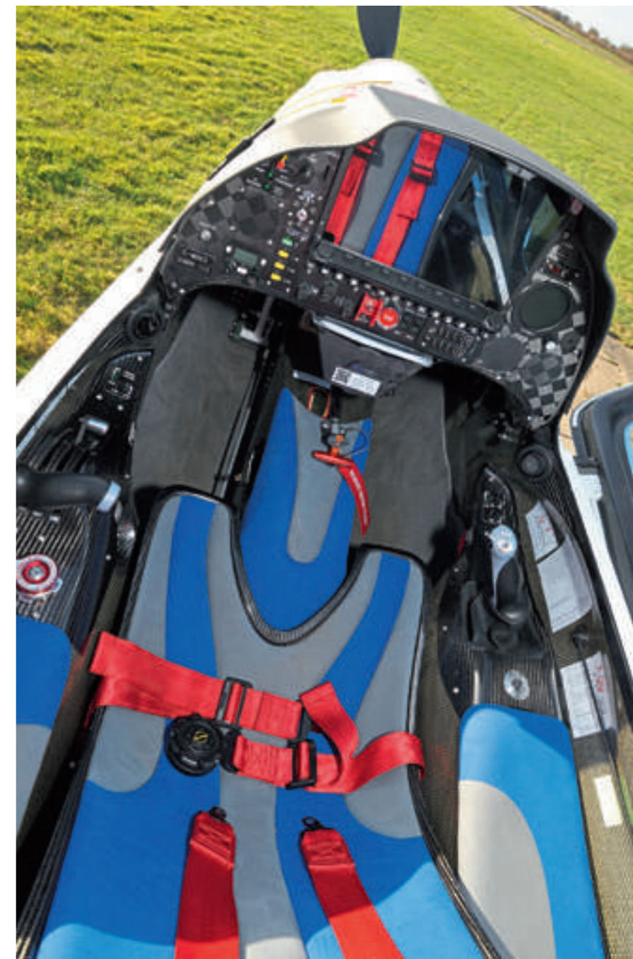
▲ Tandem reclined seats and sidesticks give the Shark a 'mini fighter' – or maybe contemporary sailplane – feel. Either way, it's just as beautifully finished
