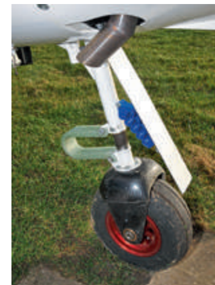
▲ Lightweight composite used for nosewheel scissor link and fork
