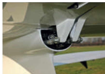
▲ Individual pushrods operate the separate elevator halves
