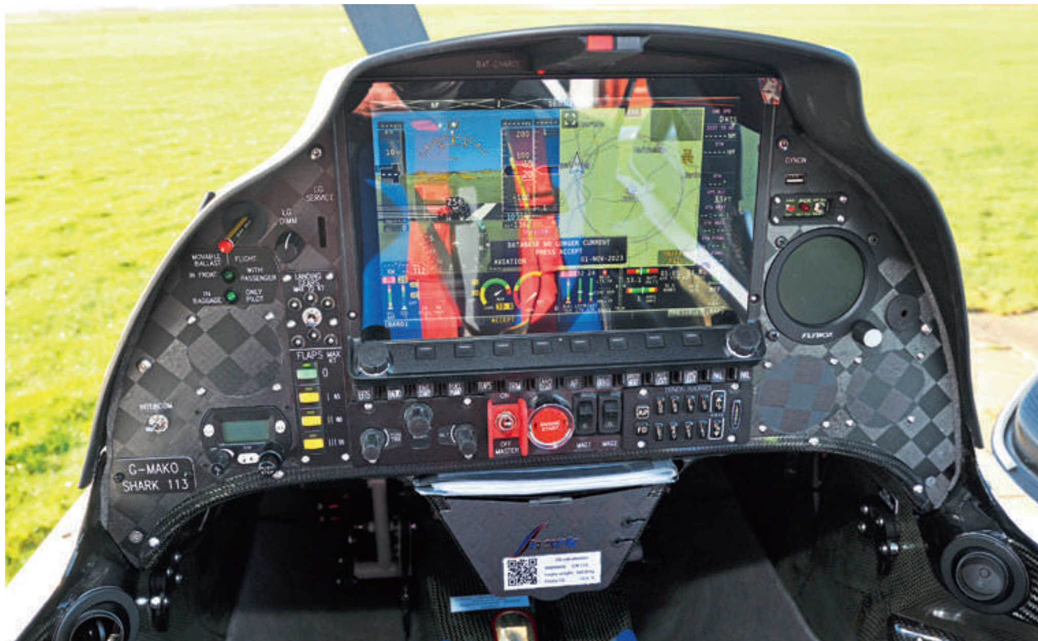
▲ Well equipped panel is dominated by the Dynon combined primary flight/multi-function display. Reliable kit, we are sure – but it is good to have a back-up combination instrument in the form of the Flybox unit (not powered up here)
