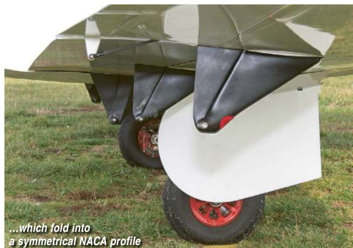
Main landing gear covers and flap suspension levers...
