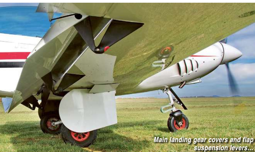
...which fold into a symmetrical NACA profile
