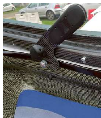
Single cockpit lock located behind the pilot's left shoulder
