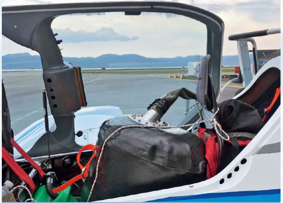
• The cockpit of the Shark with the Australian made additional tank "turtlepack" fully fuelled up
